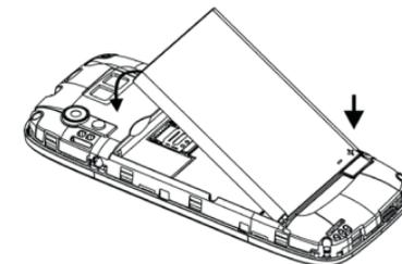
4. Lastly, put the cover back, align its tabs with the adapted slots, and gently press the cover until it snaps in place.
