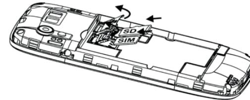
Note: Use the same process to place an external SD card in the slot located on the right of the SIM card slot.
