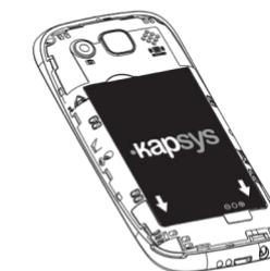
4. Lastly, put the cover back, align its tabs with the adapted slots, and gently press the cover until it snaps in place.
